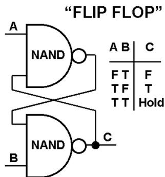
Because computer logic happens within time, “memory” circuits become necessary to hold patterns of information. A simple memory circuit, called a “flip flop,” can be constructed with two NAND gates as shown (left). Applying a “False” signal to input “A” causes output “C” to become “False;” applying a “False” to input “B” will cause “C” to become “True.” If both “A” and “B” are true, then “C” will hold (or remember) its previous status.
