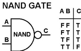
For various reasons, a NAND gate (left) is more commonly used than an AND gate in computer design. A NAND gate simply outputs the opposite, or *inverted*, state from what an AND gate outputs.
